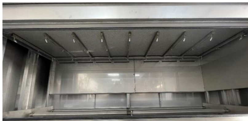
Fig.: Option: Fresh water flush with nozzle system and protective plates
