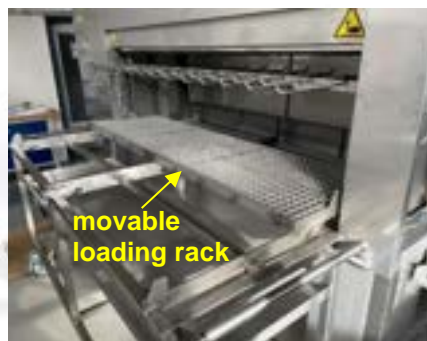
Fig.: Transport trolley with adaptable movable loading rack – here with loading rack for hooks
